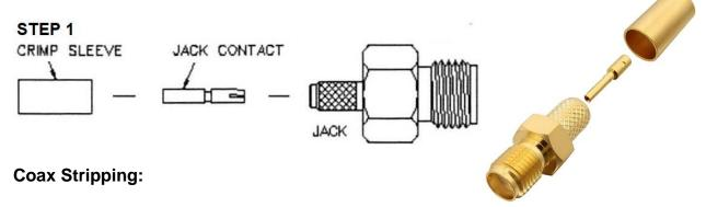
First cut your coaxial cable to the desired length and then strip the black jacket back approximately 10.5mm (0.41"). When the jacket is stripped back the dielectric 3mm (0.118") from the fresh end down to the center conductor. The braid needs to be looked at to ensure it is cut back further than the dielectric to insure that none of the braid or foil is touching the center conductor which could cause a short.
