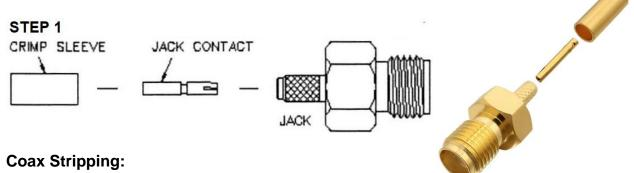
First cut your coaxial cable to the desired length and then strip the black jacket back approximately 9mm (0.35"). When the jacket is stripped back the dielectric 3mm (0.118") from the fresh end down to the center conductor. The braid needs to be looked at to ensure it is cut back further than the dielectric to insure that none of the braid or foil is touching the center conductor which could cause a short.
