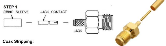
First cut your coaxial cable to the desired length and then strip the black jacket back approximately 9mm (0.35"). When the jacket is stripped back the dielectric 3mm (0.118") from the fresh end down to the center conductor. The braid needs to be looked at to ensure it is cut back further than the dielectric to insure that none of the braid or foil is touching the center conductor which could cause a short.
