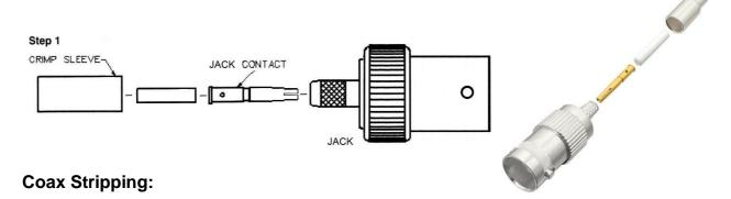
First cut your coaxial cable to the desired length and then strip the black jacket back approximately 17mm (0.67"). When the jacket is stripped cut the braid/foil back 6mm (0.236") from the fresh cut end. Finally, cut back the dielectric 5mm (0.196") from the fresh end down to the center conductor. The braid needs to be cut back further than the dielectric to insure that none of the braid or foil is touching the center conductor which could cause a short.
