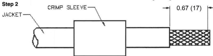
Trim back the braid 0.35 inches / 9mm from the fresh cut end. Comb out the braid and fan it out to you can get to the dielectric. Trim back the dielectric approximately 0.63 inches / 16mm from the fresh cut end.
