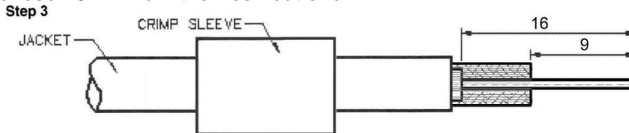
Place the dielectric spacer onto center conductor.
