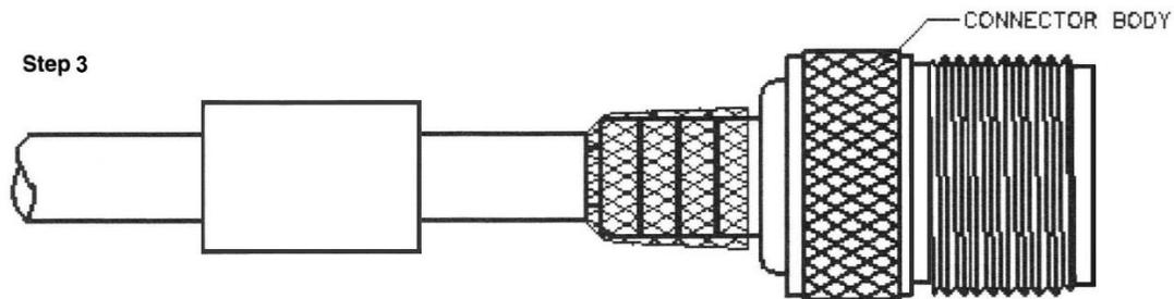
Slide the ferrule (placed on the coax at the beginning of Step 2) over the braid and completely up against the connector body. Using the 0.429 hex of the 7505-DIE-400 installed into the 7505-HANDLE ratcheting crimp handle, crimp the ferrule at the location shown in the picture below (on the ferrule, but right up against the main body of the connector).
