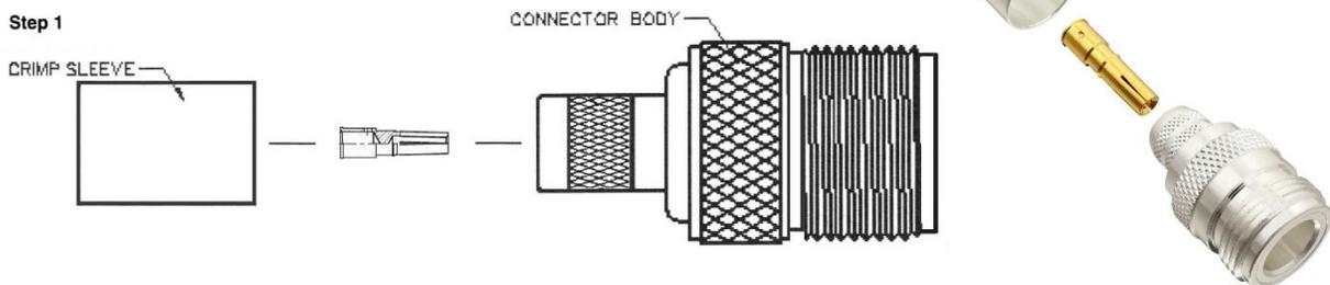
Each connector consists of one body assembly (jack), one rear ferrule (crimp sleeve), and one center pin (jack contact).
