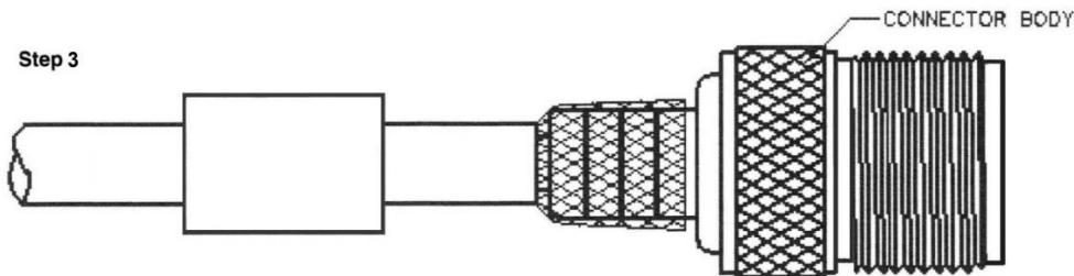
Slide the ferrule (crimp sleeve) forward and make sure it is in contact with the body assembly. Using the 0.255" hex die from the 7505-DIE-8X ratcheting crimper die to crimp the ferrule (crimp sleeve) right up next to the main body assembly. This crushes the metal sleeve around the braid and knurling to make it difficult for the connector to be removed. Trim any braid that extends out from crimp sleeve, against the body assembly, so not have any strays sticking out.
