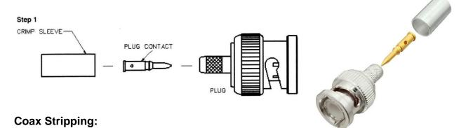
First cut your coaxial cable to the desired length and then strip the black jacket back approximately 15mm (0.59"). When the jacket is stripped cut the braid/foil back 7.2mm (0.28") from the fresh cut end. Finally, cut back the dielectric 3mm (0.12") from the fresh end down to the center conductor. The braid needs to be cut back further than the dielectric to insure that none of the braid or foil is touching the center conductor which could cause a short.
