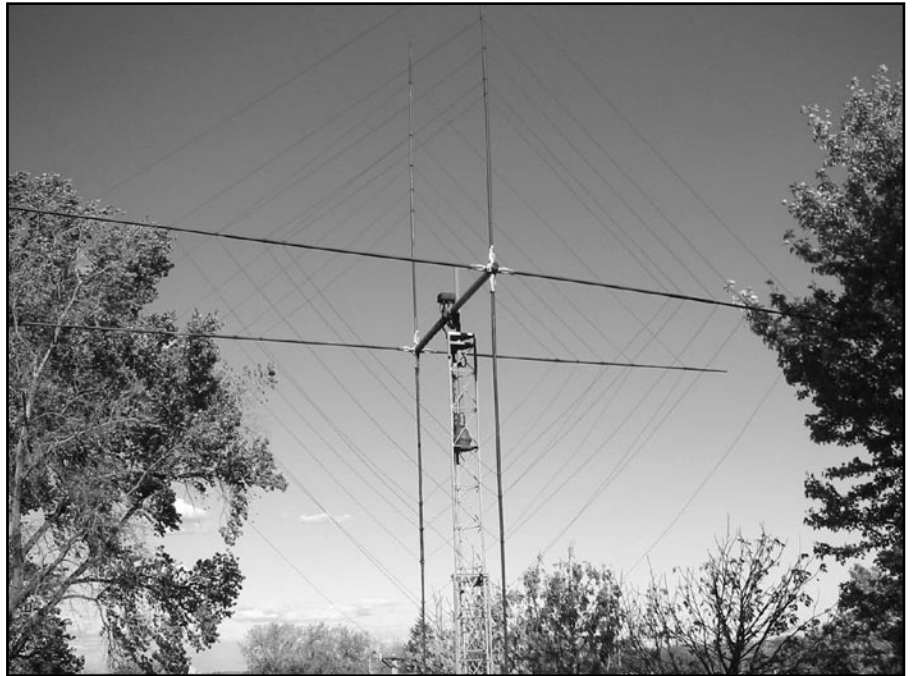
Figure 1 — Cubical quads, like this one assembled by the author, can last a long time by using the proper construction techniques.
